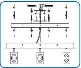
Adjust the floating canopy to position it such that it covers the j-box. Mount the back plate to the wall by inserting the supplied screws into the anchors.
