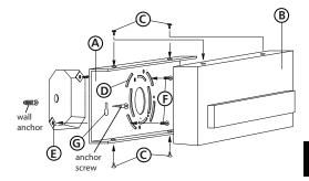
\*\*\* The construction of this fixture will be accomplished by first mounting the mounting strap to the junction box, making all necessary electrical connections, mounting the fixture to the wall, and then installing the glass.
