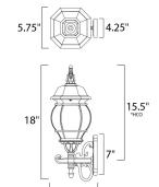
7.25' "height from center of outlet to the top of the fixture
