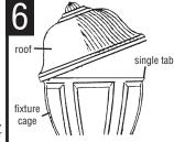
SCREW LIGHT BULB INTO SOCKET. Be sure to use bulb with wattage no greater than specified for this fixture. Lower roof and snap into place.
