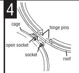
SLIP ONE HINGE PIN on roof into hole in socket on cage and snap other hinge pin into open socket
