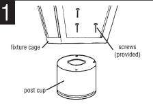
FASTEN THE CAGE to post cup with the 3 screws provided
