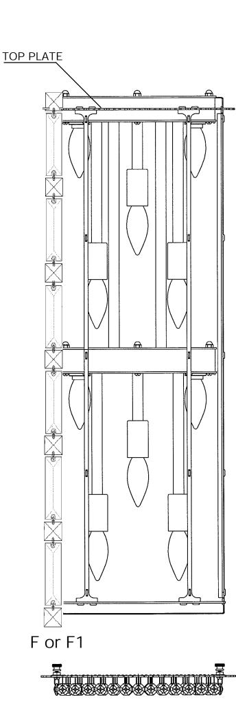
7 Install bottom crystal grid with four thumb nuts (already screwed onto grid) to bottom of the wall sconce.
