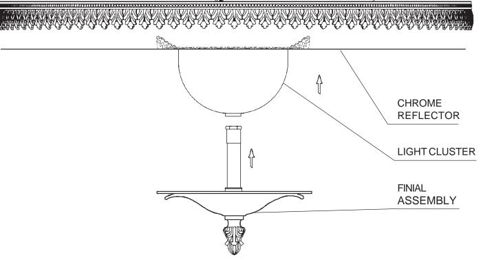
1 Remove crossbar from light cluster and reflector. Attach to outlet box in ceiling.
