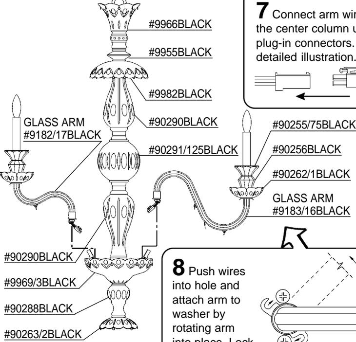
**8** Push wires into hole and attach arm to washer by rotating arm into place. Lock down by tightening screws into flange. See detailed illustration.
