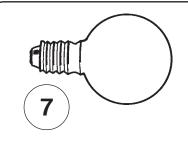
You will need 4 - G16-1/2 25 Watts Recommended 40 Watts Max MIN 90°C SUPPLY CONDUCTORS
