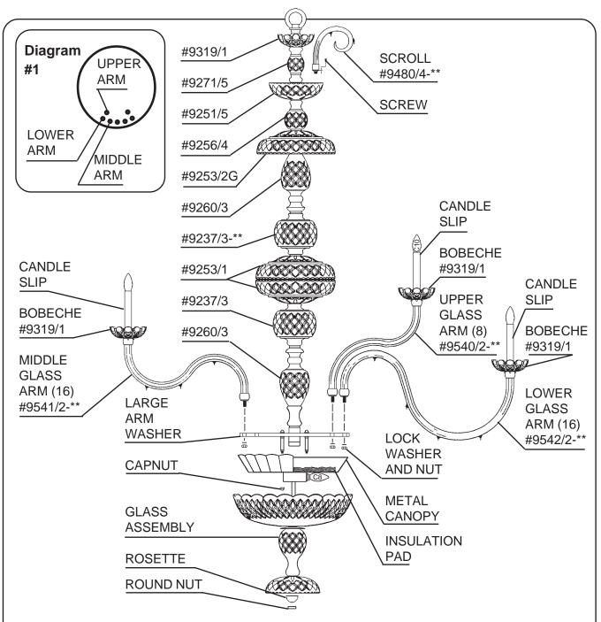
8 Install scrolls into washer with screws provided. Install arms into large arm washer. Line up holes in arms with dimple in washer. Use lock washer and nut to secure arms in place. NOTE: Place 8 upper arms into inside diameter holes and ALTERNATE 16 middle and lower arms in outside diameter holes. For best appearance line-up lower arms with upper arms. See Diagram #1.
