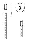
3 Cut the cable cleanly with wire cutter to desired length, and slide brass collar over wire. Position collar so that a small section (1/16") of braided wire protrudes from the top of the collar.
