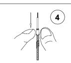
**5** Grasping the collar, slide braided outer wire back to expose inner wire. Trim 1/8" of insulation from the inner wire with wire stripper.
