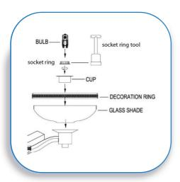
Place the glass shad the cup onto the sock Use the socket ring to
