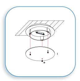
Hold the glass shade up to the canopy and secure with the supplied screws.
