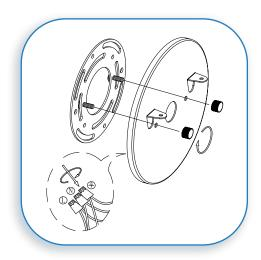
Gently pull the supply wires through the hole in the back
