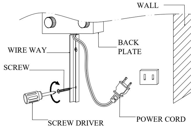
4. Attach wire way or more wire ways to be connected on the wall by screws provided.
