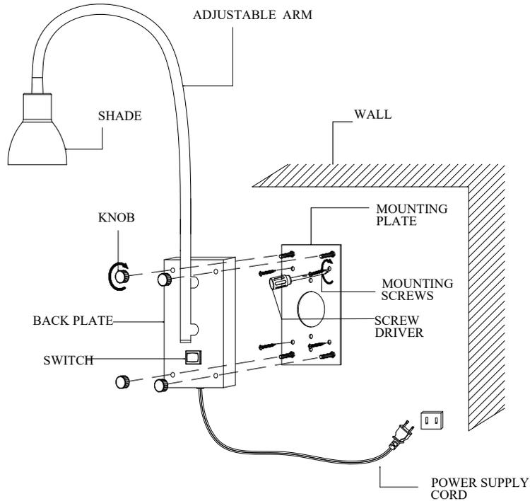
1. Unscrew 4 knobs on back plate and separate back plate from mounting plate.
