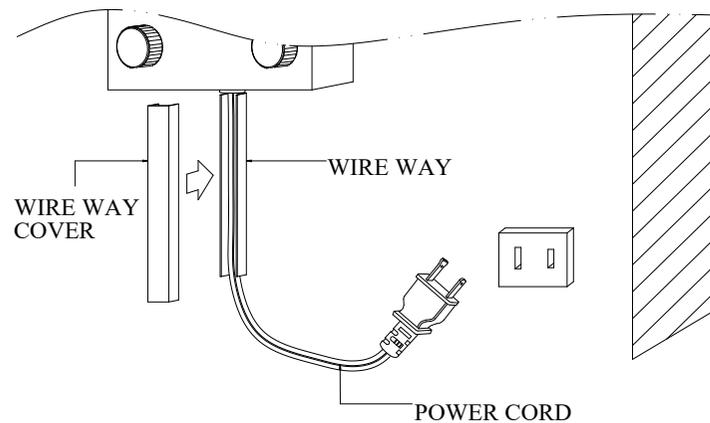
5. Push power cord inside slot of wire way and recap the wire way cover by pushing so wire way cover locks into the wire way.
