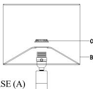
2. PUT SHADE (B) ONTO THE TOP SOCKET OF THE BASE (A) TIGHTEN IT WITH SOCKET RING (C).
