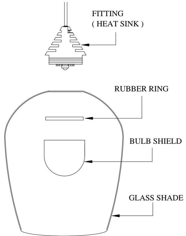
2. Put the heat sink ( fitting ) into the top hole of glass
