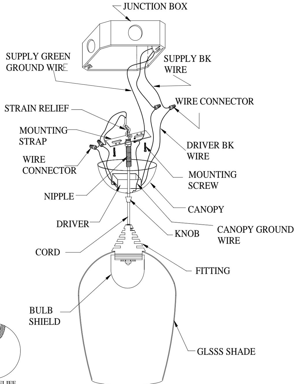
USE THE RUBBER RING TO HELPFULLY INSTALL THE GALSS BY BULB SHIELD TIGHTLY
