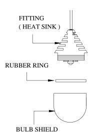
1. Remove the bulb shield and rubber ring from the heat sink ( fitting ) from the package.
