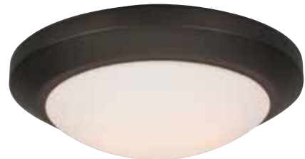
LKH2020-(FINISH)-LED - Light Kit 12.5"W x 5"H 2 - 9 Watt LED Bulbs Included 3000K Color Temp, 1500 Lumens, CRI 80 Glass: Cased Frost White Opal Finishes: BN, OB, W
