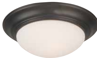
LKE53-(FINISH)-LED - Light Kit 11.0"W x 5.5"H 2 - 9 Watt LED Bulbs Included 3000K Color Temp, 1500 Lumens, CRI 80 Glass: Cased White Finishes: AB, AG, AW, BN, BNK, FB, OB, PB, W
