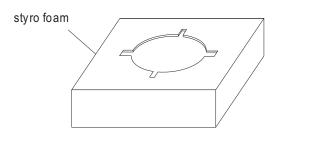
Notice:Please rest your fixture on the styro foam inside the packaging carton during the installation of the fixture in order to not damage the bottom glass leaves.
