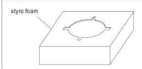
Notice:Please rest your fixture on the styro foam inside the packaging carton during the installation of the fixture in order to not damage the bottom glass leaves.
