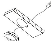
*Feed connecting cord through the hole in cabinet and secure LED lamp.*
