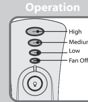
The Fan Off button only turns the fan off. To turn the fan on, press one of the fan speed buttons.
