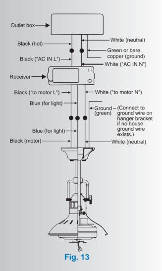
Step 2. Motor to Receiver Electrical Connections: (Fig. 13)
