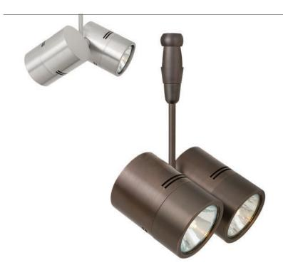
twin spot swivel Each head pivots 340°, and the entire assembly rotates 360°. Includes (2) 35 watt Halogen or (2) 6 watt LED low-voltage GU5.3 base MR16 lamps. For use with 24 volt transformer, add suffix "-24" to item number (LED lamp option not compatible with 24 volt transformers).
