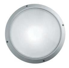
superdelta tondo visa Features an internally sandblasted glass diffuser, body and protective casing made of self-extinguishing polypropylene, aluminum reflector, and stainless steel screws. Fluorescent includes (1) 13 watt G24Q-1 base quad tube compact fluorescent lamp and electronic ballast; Incandescent accepts (1) 60 watt or equivalent E26 medium base A19 lamp (not included).
