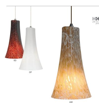
indulgent Fluted glass shade with colorful frit accents. Incandescent includes (1) E26 medium base 75 watt or equivalent A19 lamp; fluorescent includes (1) GX24Q-3 base 26 watt triple tube compact fluorescent lamp. May also be lamped with a GX24Q-3 base 32 watt triple tube compact fluorescent lamp (not included). 120v.
