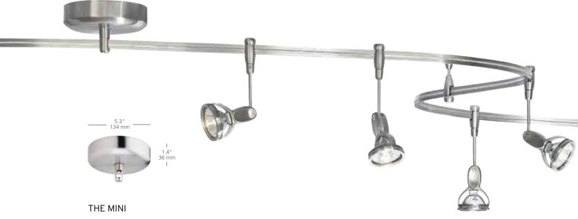
Truly minimalist design and the industry's smallest 300 watt surface transformer. Constructed of die-cast aluminum. Mounts to a standard 4" square ceiling junction box with round plaster ring (provided by electrician). To be used with special standoff specifically designed for this transformer.
