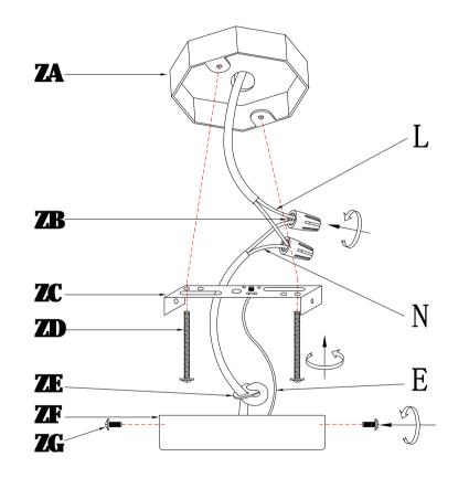
"L" = Hot wire "N" = Neutral wire "E" = Ground wire LDPD2042 D15.5"H8"L1
