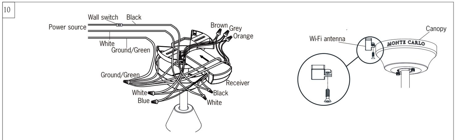
Make wiring connections using wire connectors provided as indicated above.
