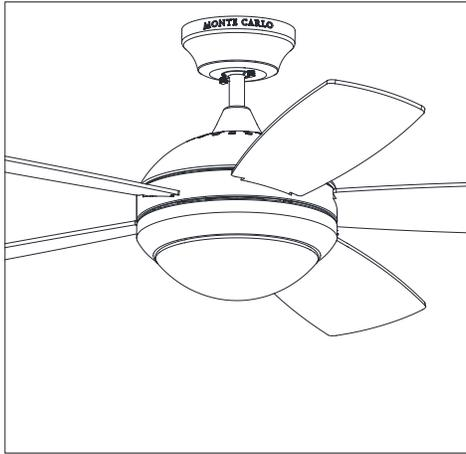
Attach light shade to the light pan by locating dimples in light pan with grooves on the light shade and twist clockwise till tight.
