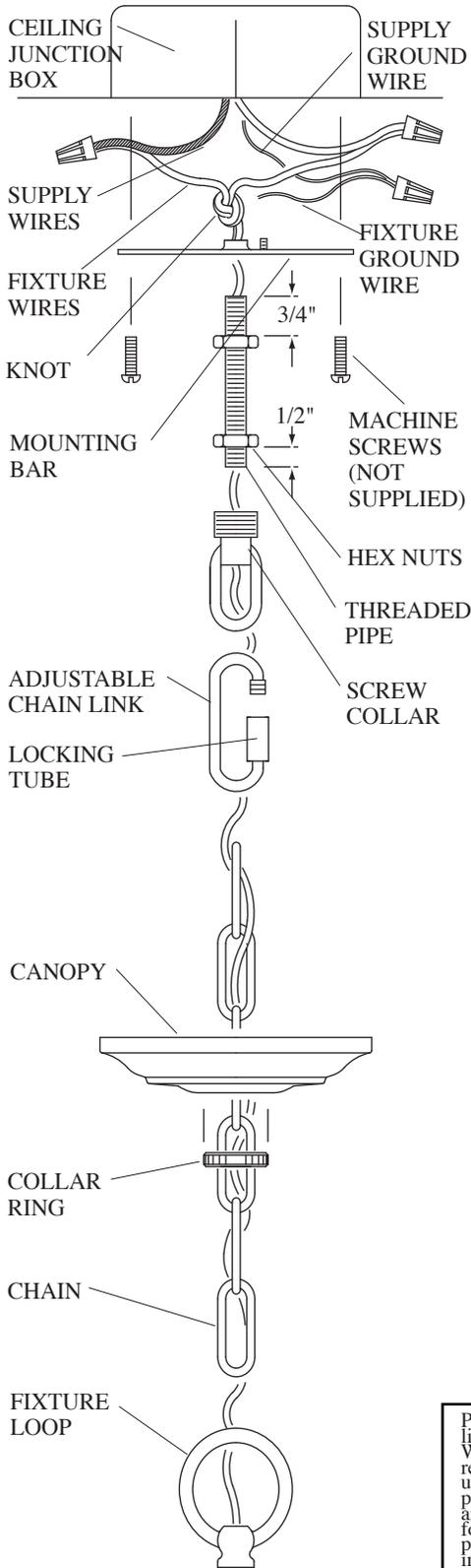
1. Attach mounting bar securely to ceiling junction box with two machine screws (supplied with junction box) through slot at each end of mounting bar. Note: mounting bar should be installed with "GND" imprint and/or two dimples facing down.
