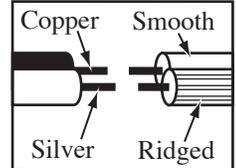
Note: Make certain no loose conductors protrude outside of wire connectors. And make certain all wires are securely held together by wire connectors.
