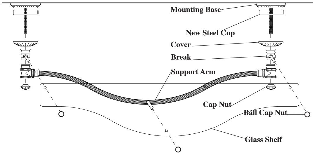
1. Hold each mounting base, (with Steel Cup removed) on desired wall location and mark locations of both holes in center of mounting base. Make sure the two sets of vertical dots are leveled to each other.
