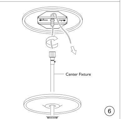
6. Install center fixture onto ceiling outlet box:
