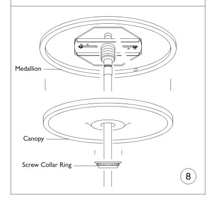
8. While gently tucking all fixture wires inside, raise canopy against the medallion and lock into position by screwing collar ring onto screw collar.
