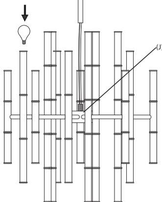
**Caution when using a wall dimmer:** To avoid a risk of fire do not exceed the maximum wattage output of the dimmer. A dimmer rated at least 750 watts is recommended for this fixture when using 25 watt bulbs.
