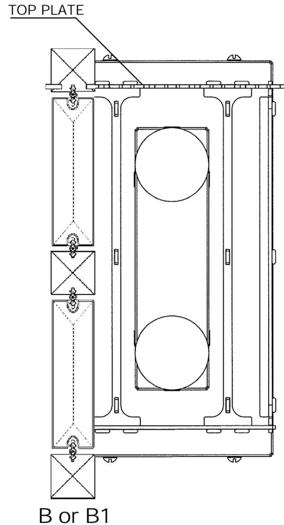
7 Install bottom crystal grid with four thumb nuts (already screwed onto grid) to bottom of the wall sconce.
