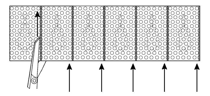
NOTE: Work on one crystal set at a time. Follow the black line from top to bottom according to the numbered steps on the trim diagram.
