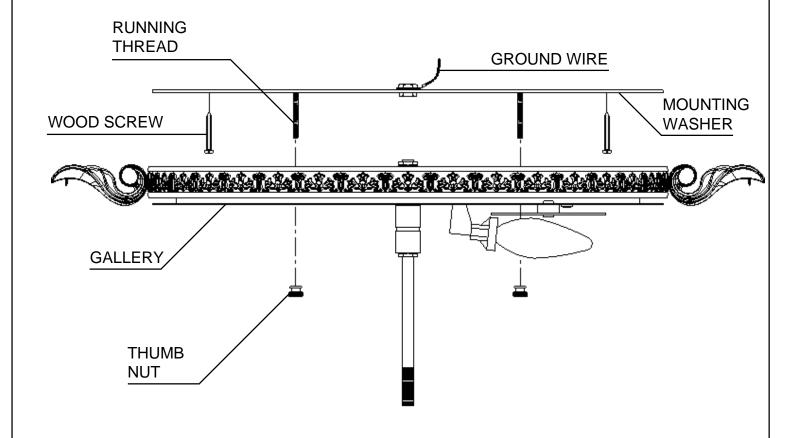
3 Attach mounting washer to outlet box. Install wood screws provided into ceiling for added support. Connect ground wires from fixture and mounting washer to ground wire in outlet box. Fixture must be grounded. Connect neutral and power wires from fixture to neutral and power wires in outlet box.
