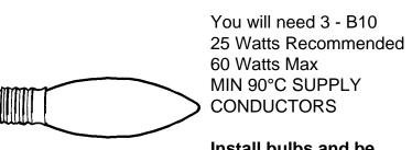
Install bulbs and be sure to test fixture BEFORE trimming.
