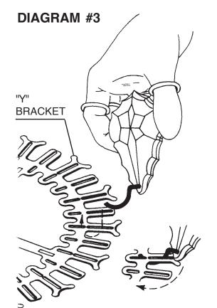
Position the crystal above the "Y" bracket so that the end of the hook enters the long slot, gently push toward the center of the fixture and raise the crystal making sure that the end of the hook comes up through the short slot, in line with the long slot.
