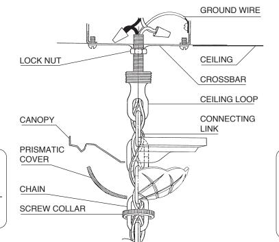
**5** Insert stem wire through chain and ceiling loop. Connect wires. Fixture MUST be grounded.
