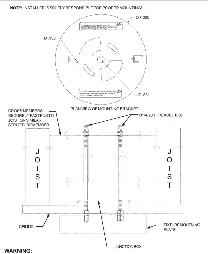
MOUNTING CONFIGURATION AND HARDWARE MUST HOLD 4X THE WEIGHT OF THE FIXTURE. MOUNTING DESIGN AND FIXTURE INSTALLATION SHOULD BE CONDUCTED BY A QUALIFIED LICENSED PROFESSIONAL.
