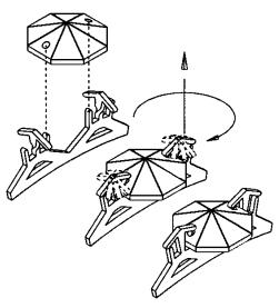
**B** Slide crystal octagon into pocket. Turn both tabs clockwise back to original position to hold the octagon in place.
