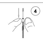
**5** Grasping the collar, slide braided outer wire back to expose inner wire. Trim 1/8" of insulation from the inner wire with wire stripper.
