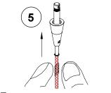
**5** Feed inner wire into quick connect adapter until it reaches top set screw. Feed braided outer wire and brass collar into quick connect.
