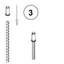
**3** Cut the cable cleanly with wire cutter to desired length, and slide brass collar over wire. Position collar so that a small section (1/16") of braided wire protrudes from the top of the collar.
