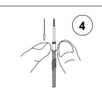
**4** Grasping the collar, slide braided outer wire back to expose inner wire. Trim 1/8" of insulation from the inner wire with wire stripper.
