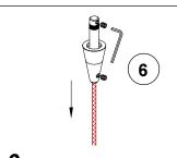
**6** Tighten top set screw first, then lower set screw snugly. Smooth out any bulges in braided wire.
