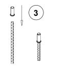
3 Cut the cable cleanly with wire cutter to desired length, and slide brass collar over wire. Position collar so that a small section (1/16") of braided wire protrudes from the top of the collar.
