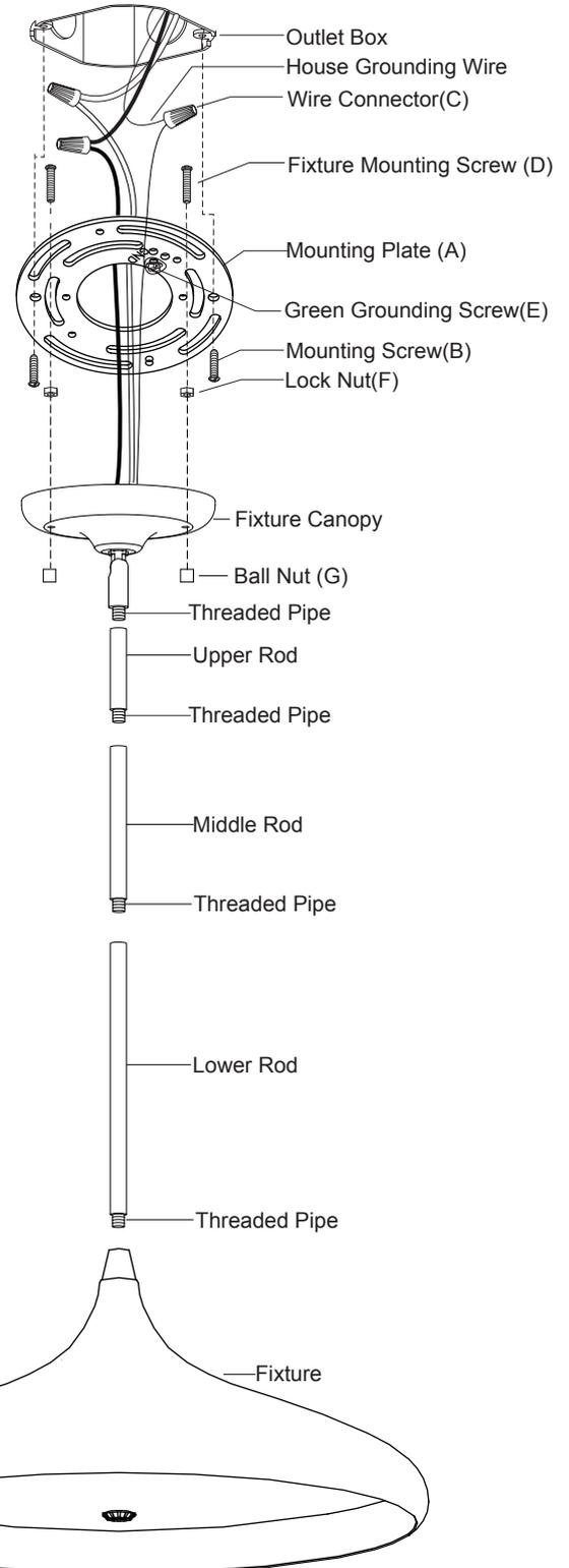
4. Pull out the source wires from the outlet box. Make wire connections using wire connectors as follows:
