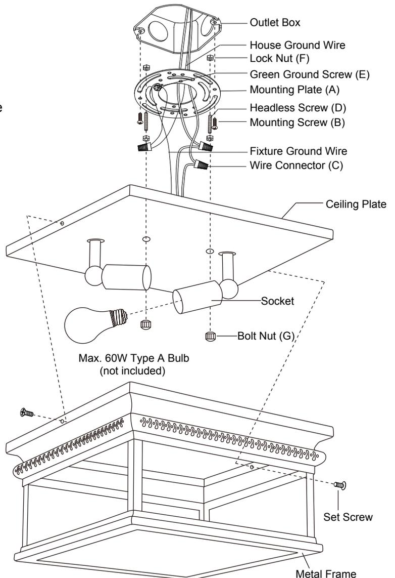
5. Install two bulbs (not included). See relamping label at socket area or packaging for maximum wattage allowed.
