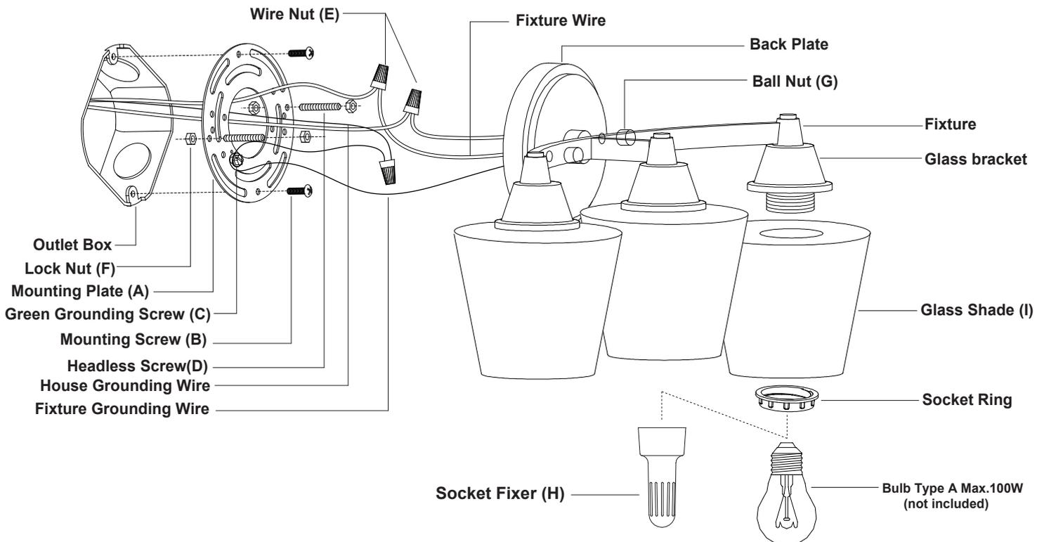
1. Thread two headless screws through the mounting plate, then secure them with four lock nuts (two on each side of the mounting plate). Adjust the length of the headless screws if necessary.
