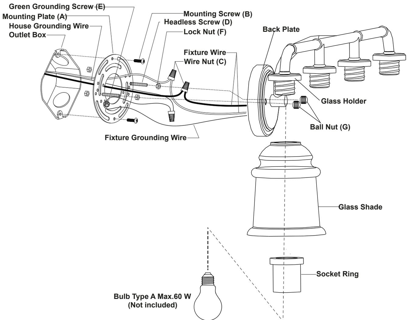
1. Thread two headless screws through the mounting plate, then secure them with four lock nuts (two on each side of the mounting plate). Adjust the length of the headless screws if necessary.
