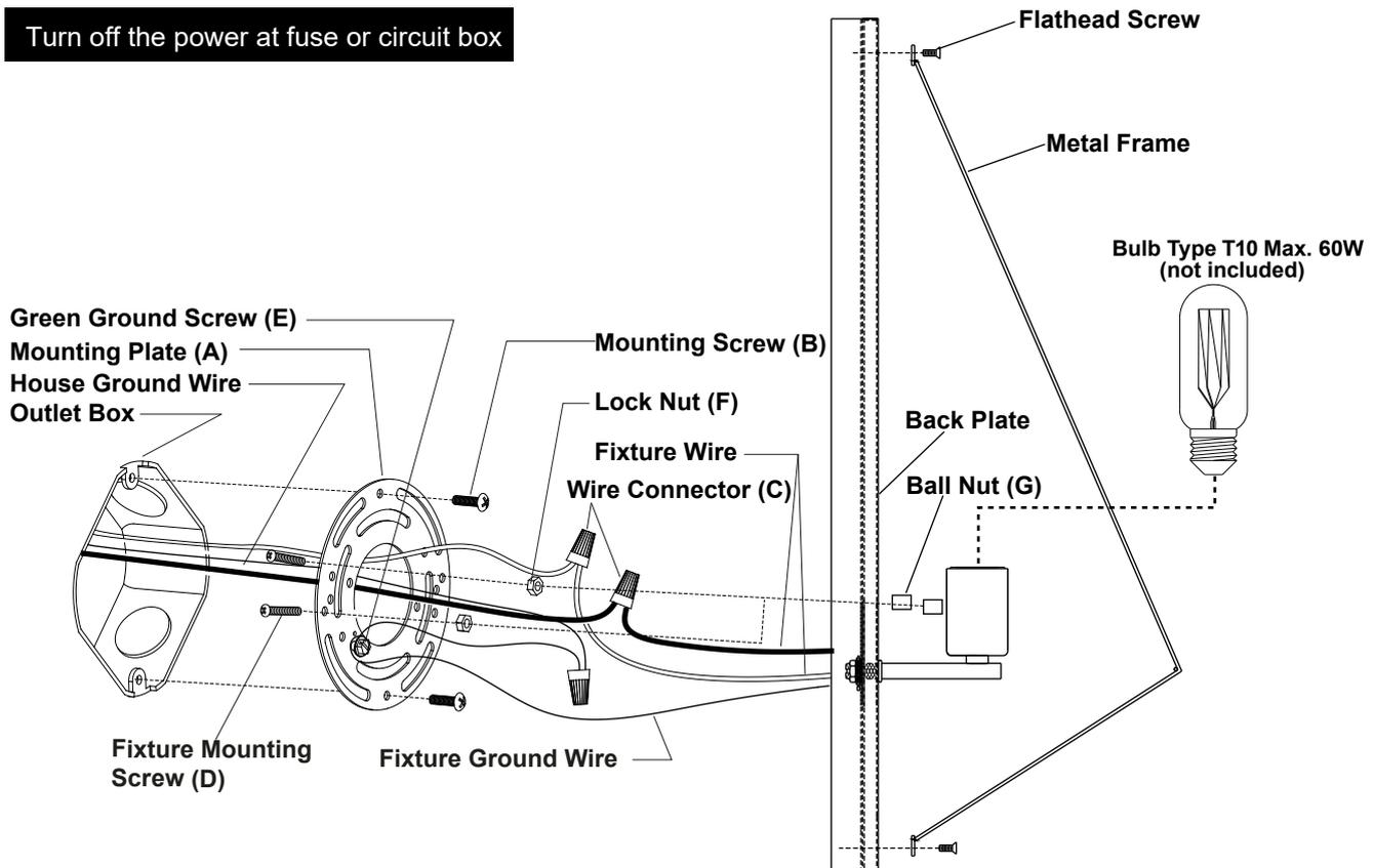
1. Attach the metal frame onto the fixture light and tighten it with the flathead screws.
