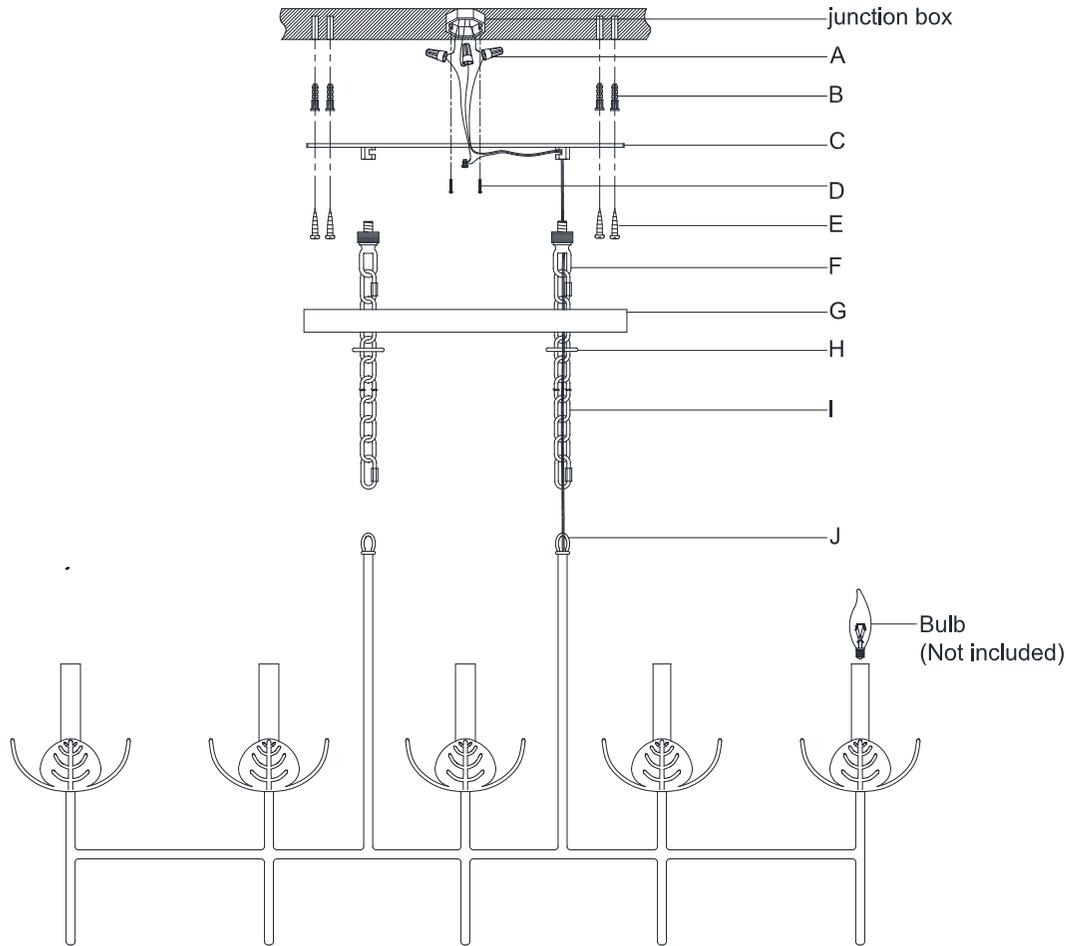
15. Connect the fixture ground (bare) wire with the ground wire from the junction box using wire nut (A). If your house does not have ground wire, then attach this wire to the green grounding screw inside of the junction box.
