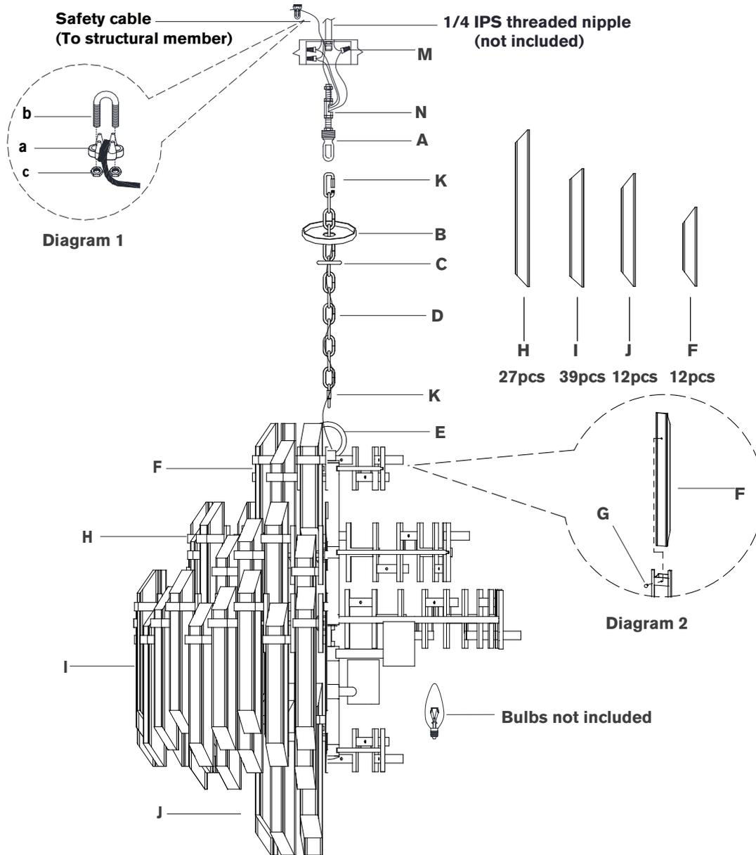
19. Carefully slide acrylic part all the way down channel on frame and secure with thumbscrew (**G**) once lined up with small divot on back. (See diagram 2)
